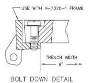
CAUTION: DO NOT DISASSEMBLE BOLTED GRATES BEFORE SETTING SECTIONS IN CONCRETE
